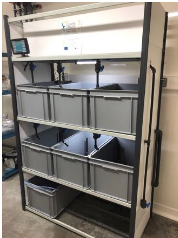
Figure 9: 50L tank version (with 6 replicate tanks) of the gravity-based tidal simulator.
