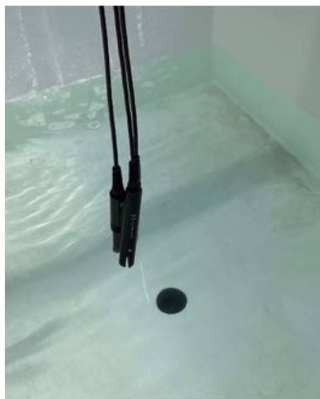
Figure 22: Temperature, salinity, pH and dissolved oxygen sensors in one of the experimental tanks.
