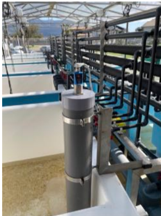
Figure 2: Ultrasonic sensor for water level monitoring.
