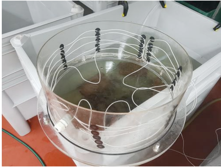
Figure 18: Prototype benthic chamber for heatwave experiments
