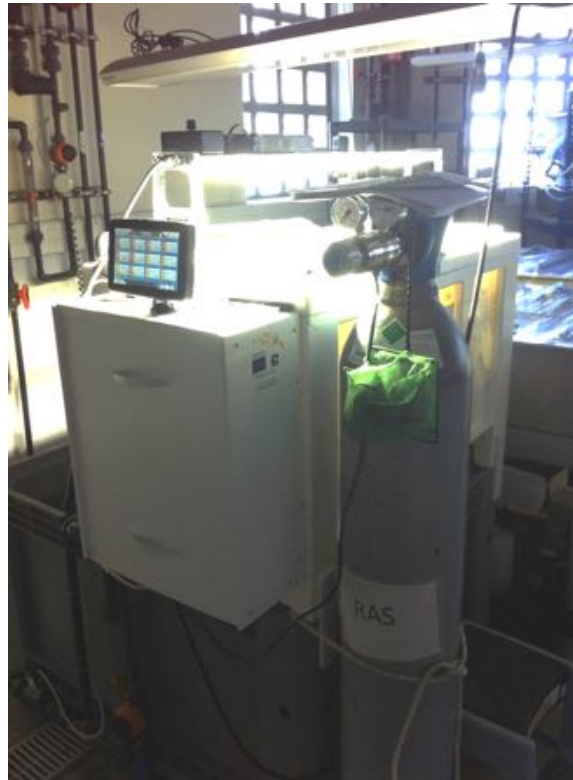
Figure 8: 300L tank version of the gravity-based tidal simulator with pH control.
