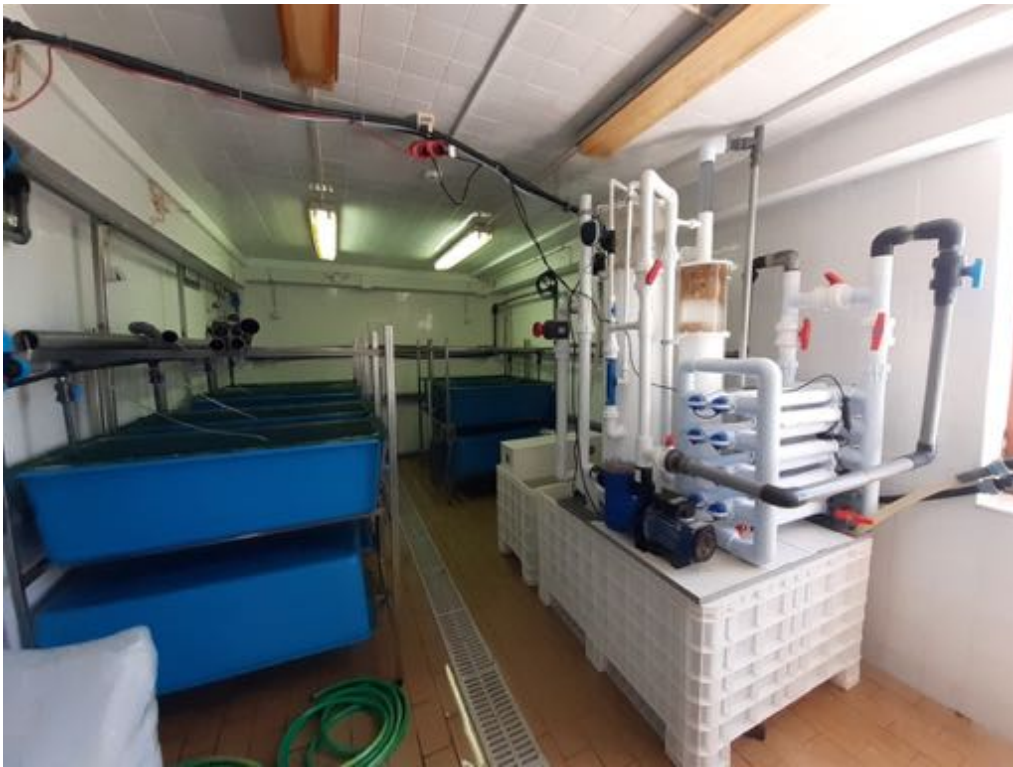
Figure 30. Raceway system for forced swimming experiments
