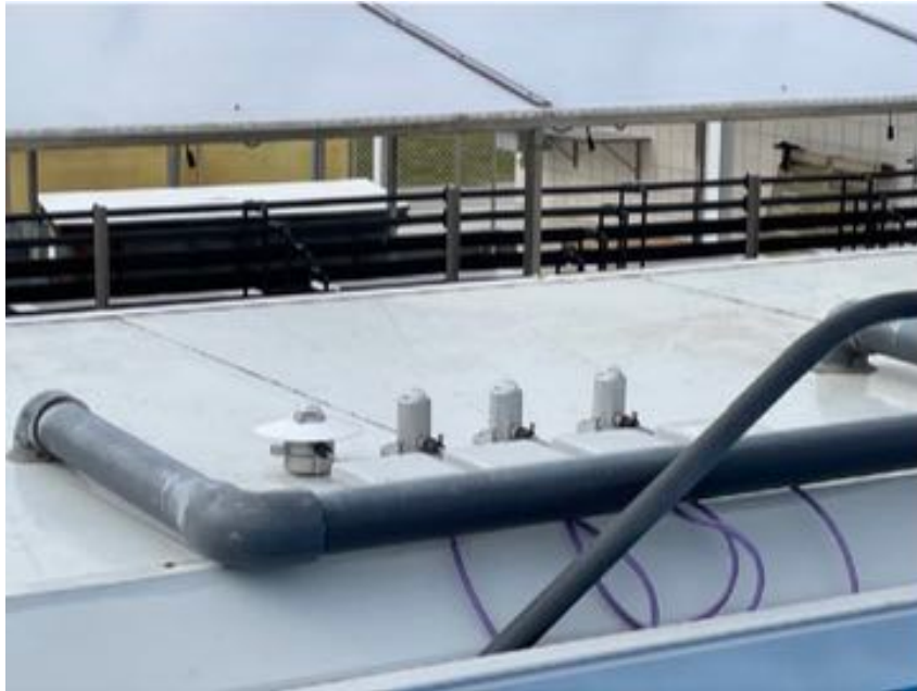
Figure 23. Sensors for global radiation, PAR, UV-A and UV-B in the ECIMAT mesocosm facility.
